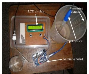
Fig.3: The pH mesurement setup
