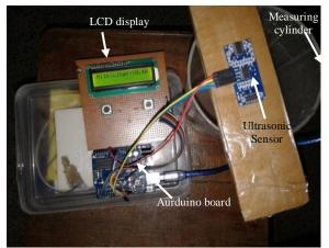
Fig.2: Milk quantity measurement setup
