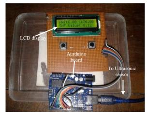
Fig 4: The CLR and SNF measurement setup
